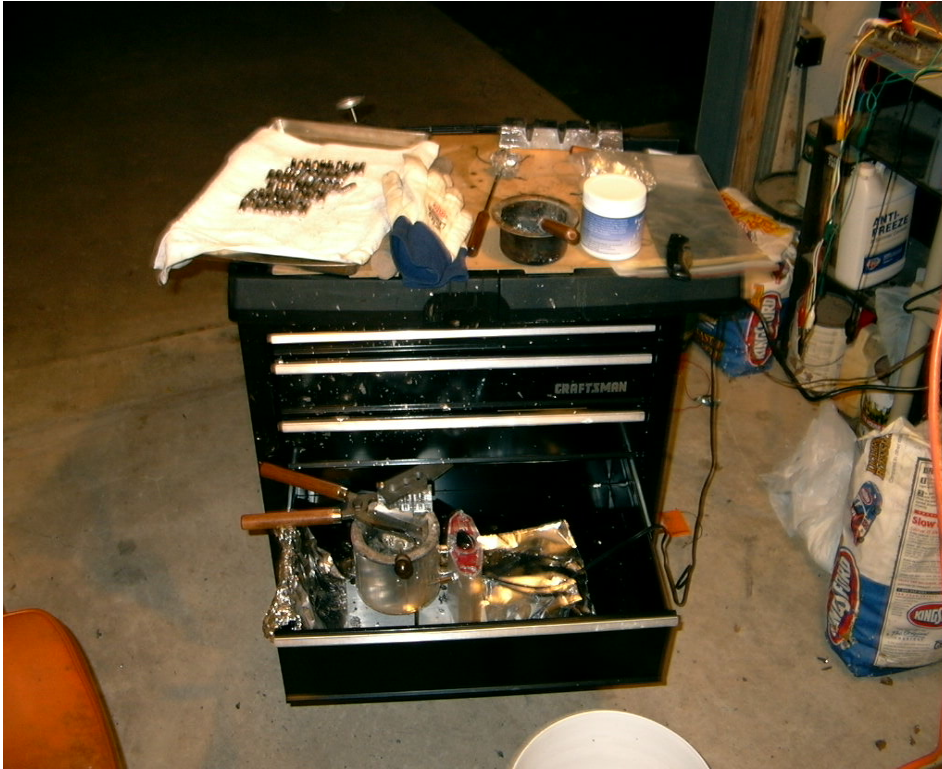
Lead Furnace with ladle and preheating of the casting mold. Tin Foil is used to catch lead splash.
