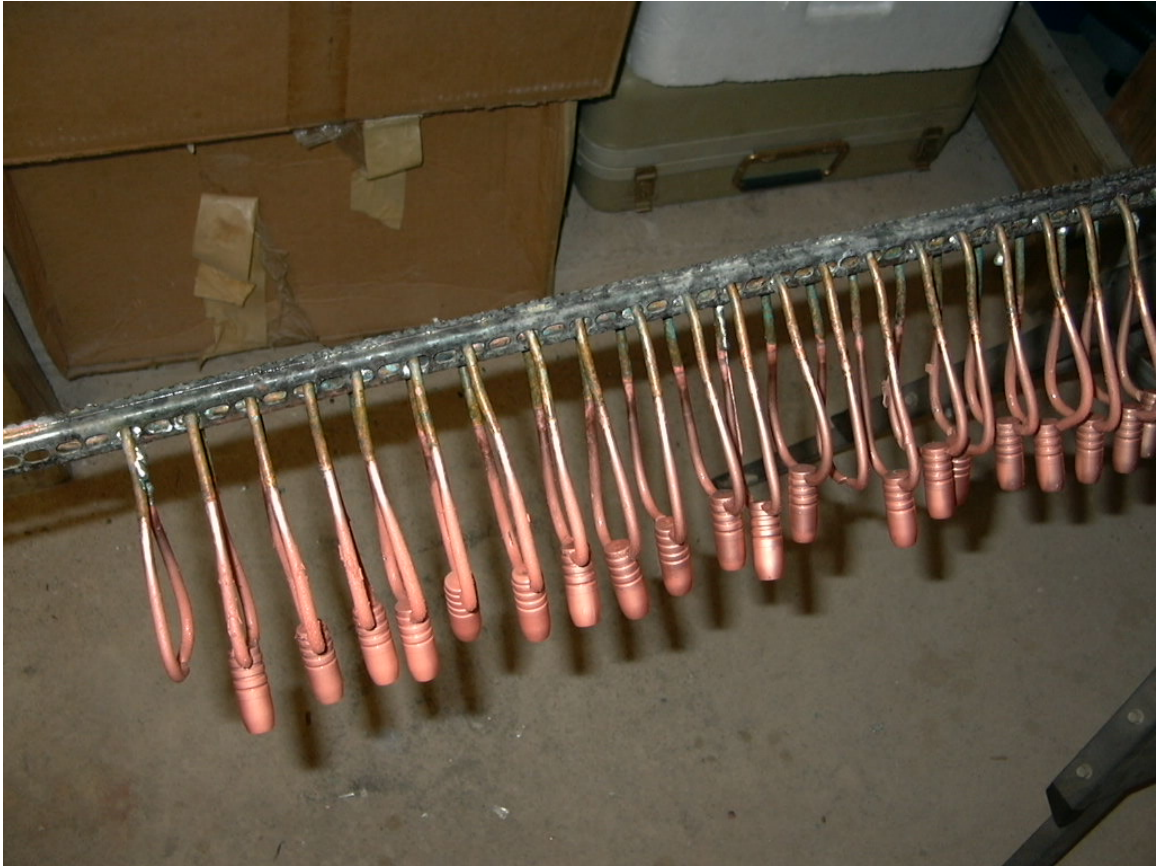
Bullets after removal from the plating process prior to polishing.
