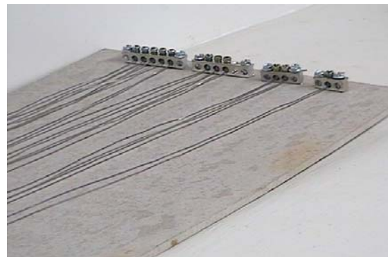
Connectors cut up and bolted to panel
